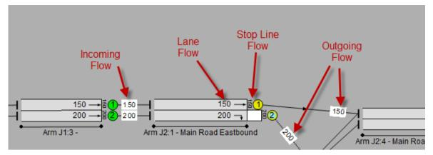
Where Flows are displayed by Layer each Layer Flow is shown in the colour of the Layer it is on. Layer colours are defined using the Edit Layers dialog box which is opened by choosing 'Edit Lane Based Flow Layers' from the Traffic Flows menu.
