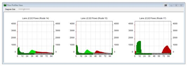
Viewing separate profiles is sometimes useful when analysing a complex model and trying to identify the effects of different signalling arrangements on different traffic movements rather than on the Lane as a whole.
