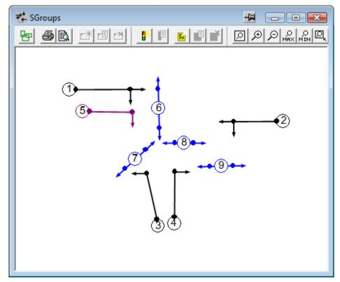
• **UK Stage View becomes Phase View.** The Phase View shows the Phases defined for each Phase Stream in a Controller. The Phases are named alphanumerically and can have alternate Phases defined.
