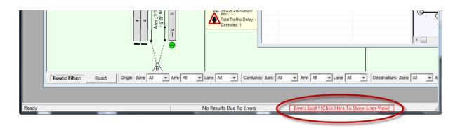
When Errors or Warnings exist in the Error View LinSig will highlight this by displaying a red or amber Error Indicator in the Status Bar at the bottom of the Main Window. The Error View can be opened by double clicking the Error Indicator.
