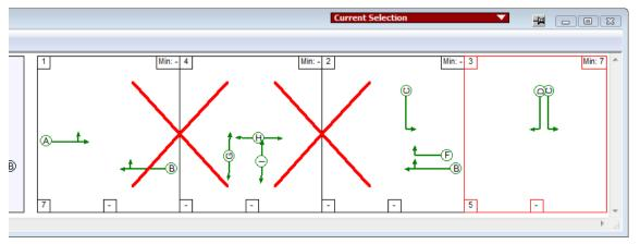
As you build up a Stage Sequence the unfinished sequence will usually show a number of sequence errors. This is quite normal and reflects the fact that the Stage Sequence is not valid until it is complete.
