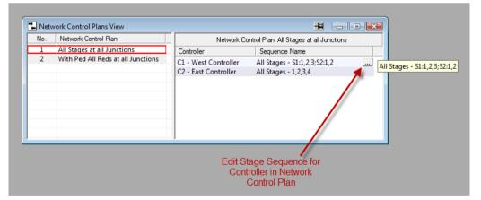
• Select a Stage Sequence from the drop down list. This is the Stage Sequence which LinSig will run for this Controller when this Network Control Plan is used in a Scenario.
