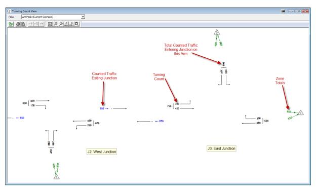
The Flow Group for which Turning Counts are displayed can be selected in the Turning Counts View toolbar. The selected Flow Group is linked with the selected Flow Group used by the Matrix Estimation View so both Views always show traffic flow information for the same Flow Group.
