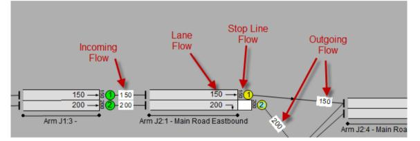
• Lane Based Flow Tabs of the Edit Lane Dialog Box. The Edit Lane dialog box provides one or more tabs which allow detailed editing of Lane Based Flows on a Lane. This method is simply an alternative non-graphical method of entering the same data as the graphical method.
