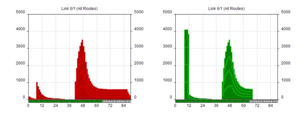
Each Route Flow Profile is shown as a separate 'layer' in the graph. The layered Route Flow Profiles cannot be shown on a combined inflow/outflow graph as the display becomes extremely complex and difficult to understand.
