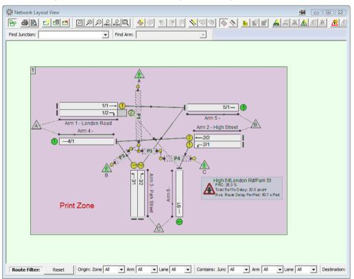
As shown in above a Print Zone is a rectangular area of a View and defines the content that will be included on the printed page corresponding to the Print Zone. Any number of Print Zones can be defined, with each Print Zone corresponding to a Printed Page.
