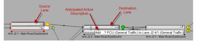
Release the mouse button while pointing at the Destination Lane. LinSig will display the 'Specify Lane Based Flow Details' dialog box which allows detailed settings for the Lane Flow being entered to be specified.
